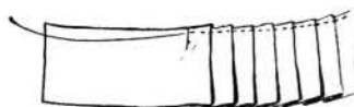
Diagram 4. Ribbon side plaited for ruffle. Use twice as much material as space covered.
