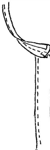
Fig. (40) The collar facing turned onto the wrong side of the garment
