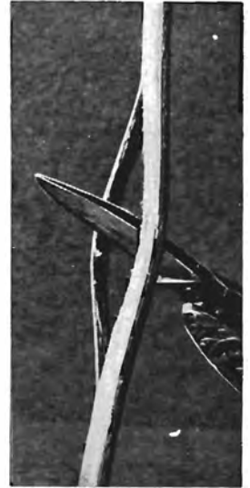
FIG. 2. MAKE AN INCISION IN A SPOKE
